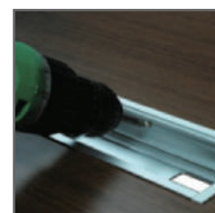
Drill holes on the table according to the pre-drilled areas of the housing and tighten the self-tapping screws secure the housing
